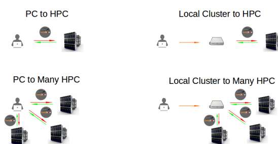
Figure 2: Modes of operation of the Longbow job submission tool. Longbow can connect to one or more remote HPC resources, and can be run on a laptop/desktop or as part of a longer workflow on a local cluster.
